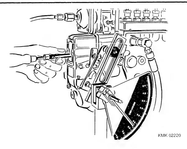
GOVERNORS WITH MANIFOLD—PRESSURE COMPENSATOR (LDA) AND BUILT—IN FULL—LOAD STOP
